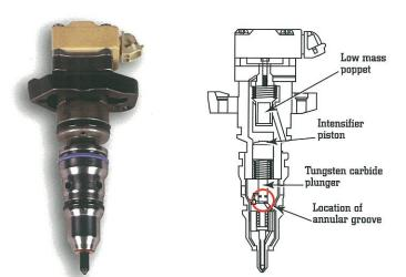
A new injector has been released with the following changes:
