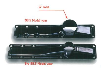
Both the Econoline and the "F" Series use a new intake cover with 3" inlets into the heads for better flow to the combustion chambers. The new cover has had no modifications to length or bolt pattern. With this change, the CAC to intake hoses are now straight with 3" diameters on both ends. These hoses have no hump between the two components. On the non charge air cooled Econoline engines, an aluminum "Y" pipe with 3" inlets and outlets is now used.
