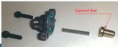
If a leak occurs at the high pressure oil gallery plug, a service plug for the high pressure oil rail that places the sealing o-rings deeper into the gallery is now available. The new plug can be identified by a circular groove cut into the face of the plug. The new plug went into production prior to 1999.5 MY on engine S/N 751869.
