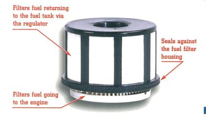
During the 99 model year a dual element fuel filter was incorporated to filter the fuel that is returned to the tank via the fuel filter regulator. The Ford Replacement Part Number for this filter is unchanged: F81Z-9N184-AA.
