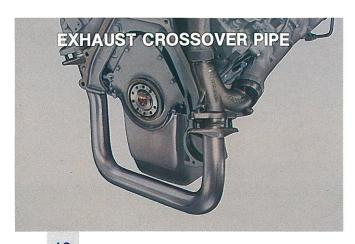
Figures 17, 18 & 19 identify external features of the 7.3L IDI Turbocharged Diesel Engine. Included are the air cleaner assembly, turbocharger assembly and crossover pipe.
