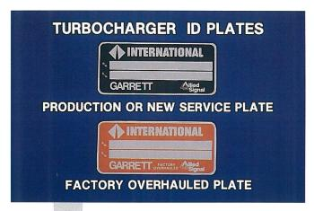
The part number of the turbocharger should always be verified whenever replacement is performed by comparing part numbers on the name plates.
