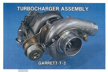
The Garrett T-3 turbocharger allows the engine to operate up to 10,000 ft. elevation with no loss of power. Intake manifold pressure (boost) will be modulated through the use of a wastegate.
