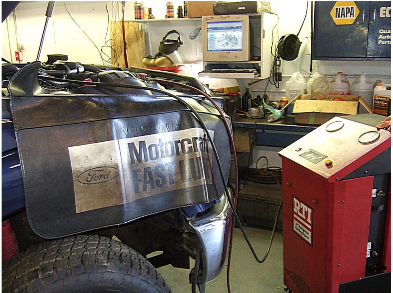
While the cooling system is draining, I evacuate the air conditioning.
