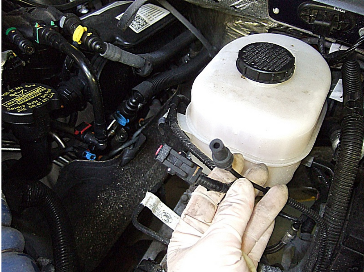
This vehicle is equipped with automatic four wheel drive and the hub lock solenoid is mounted on the degas bottle. I disconnect the solenoid wiring and vacuum supply hose and remove the degas bottle.
