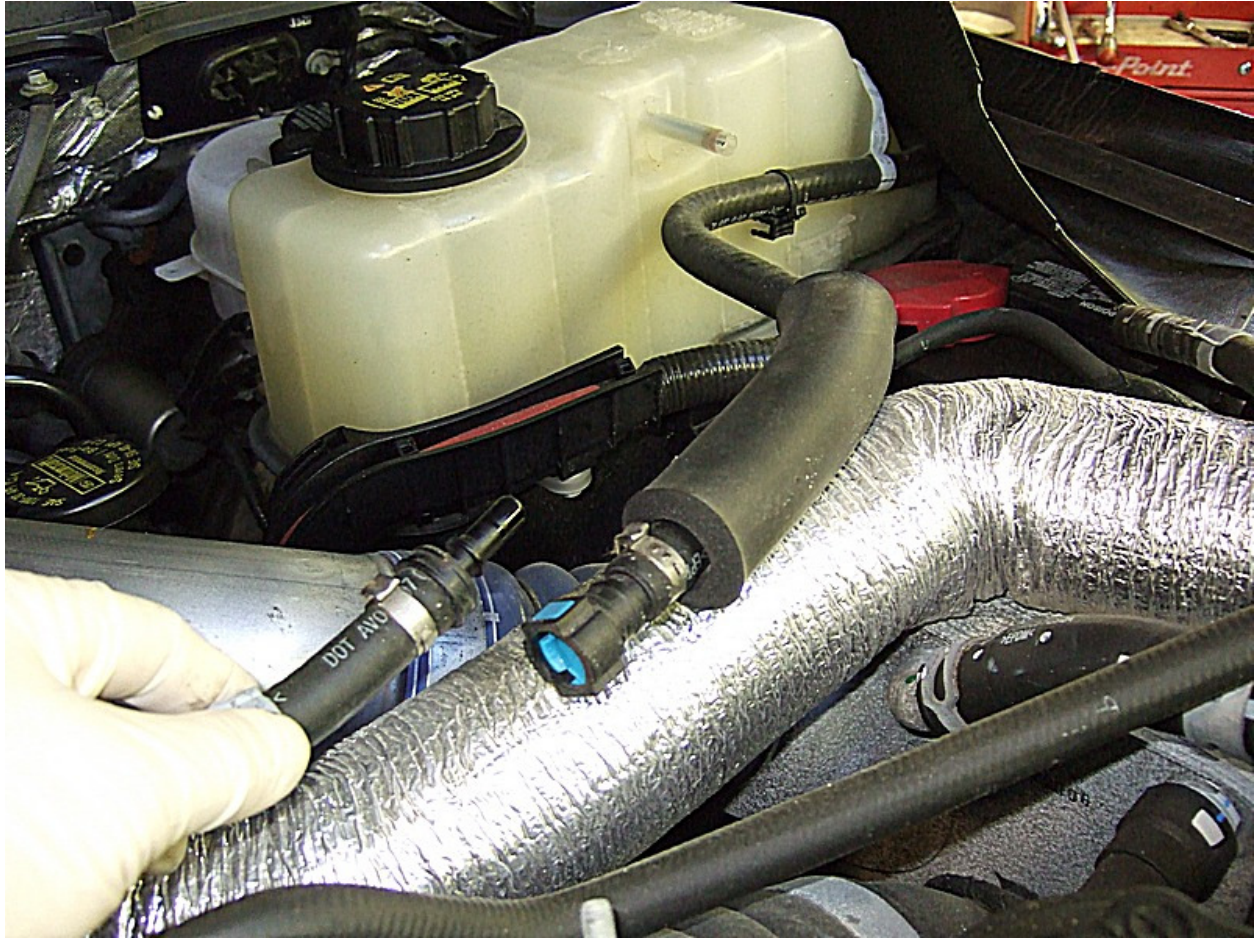
This is the vacuum supply line from the vacuum pump.
