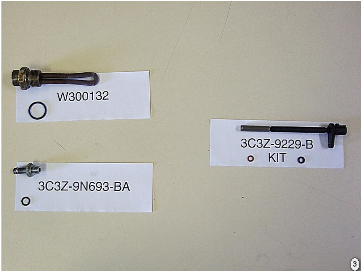
The block heater "o"-ring is a 4ct., cam "o"-rings is a kit, oil drain back fitting "o"-ring.
