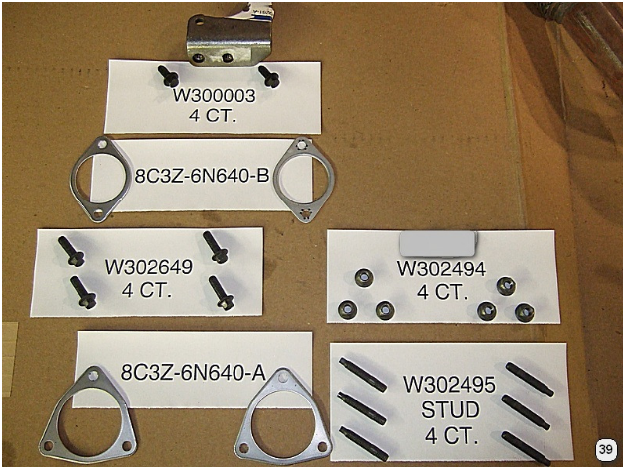
Turbo up pipe bolts and gaskets.
