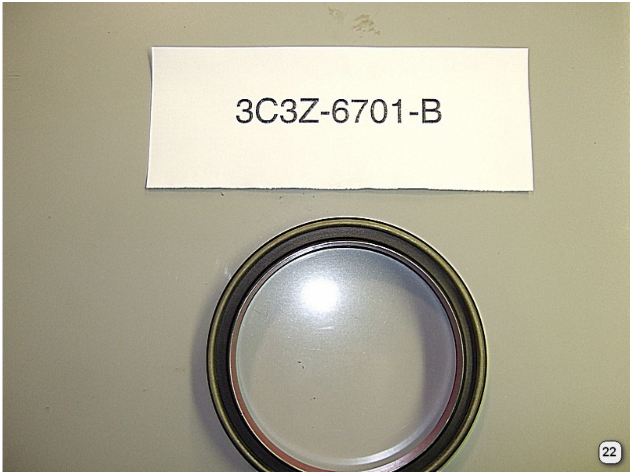
Updated rear main seal with full sleeve and loc-tite preapplied.
